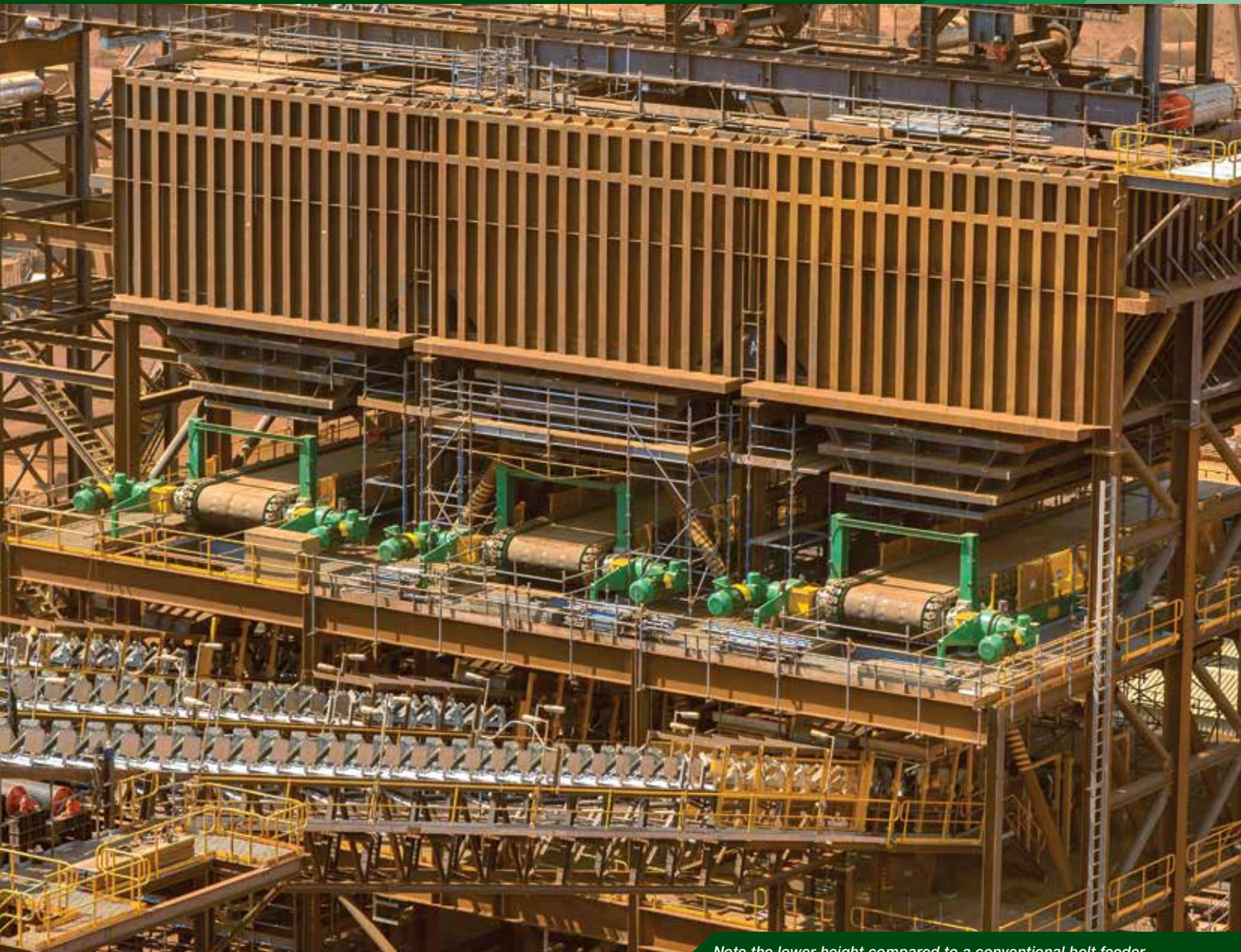
Note the lower height compared to a conventional belt feeder.
