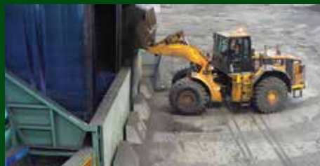
Bulk loading and unloading hoppers are ideal for reclaim via front end loaders.
