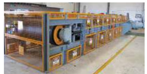
Hydraulic assisted tensioning.
