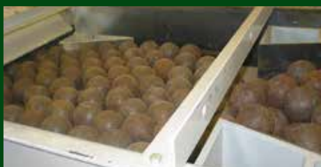
Ball storage capacities to suit mill usage and various ball diameters (27 - 150mm).
