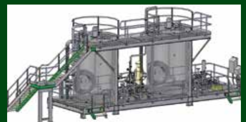
Typical Transmin reagent mixing and storage facility, designed and supplied as a stand alone module.
