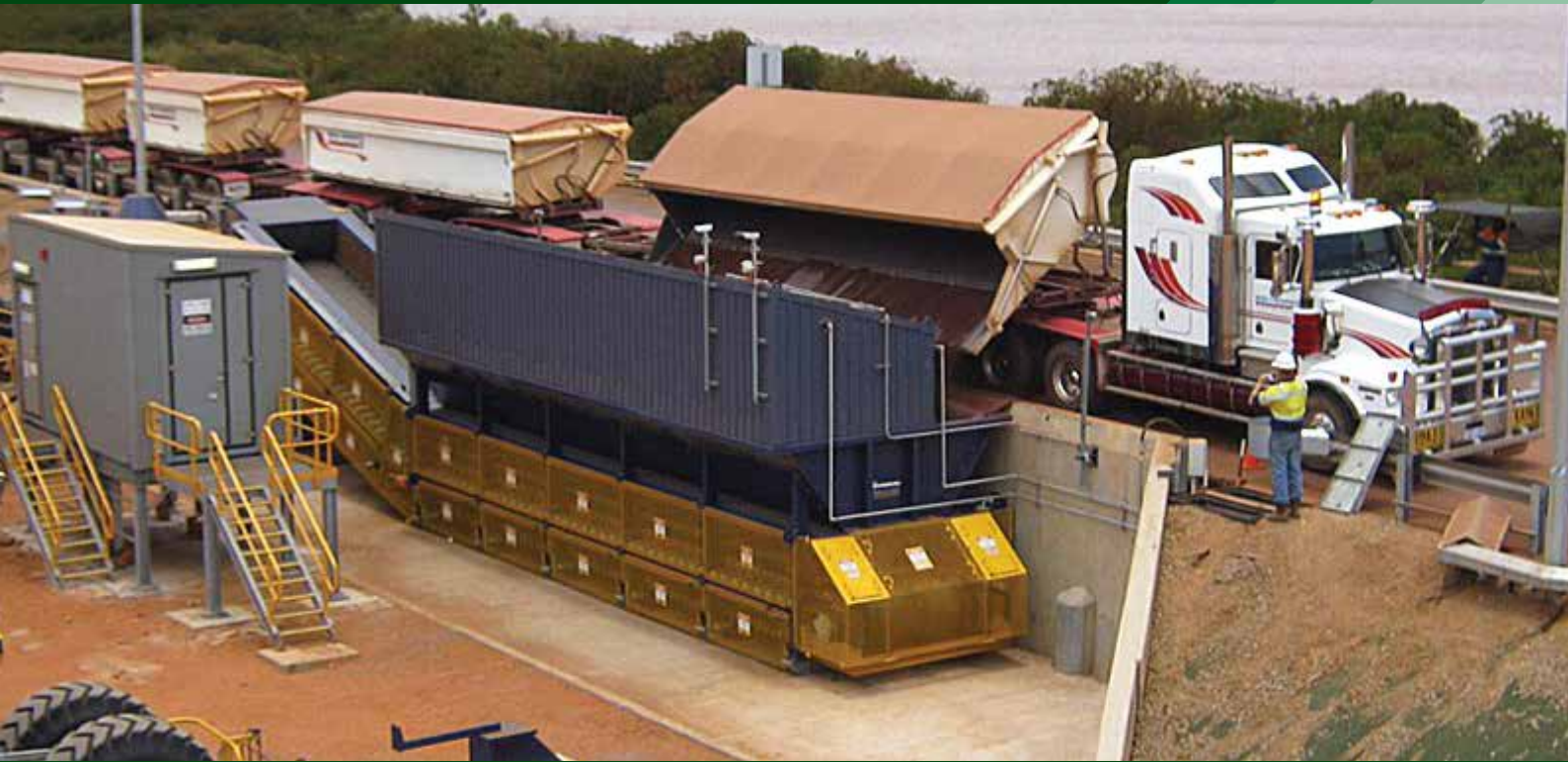
Direct rail wagon – receipt and transfer
