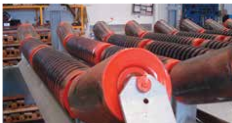
Impact idlers for load support.
