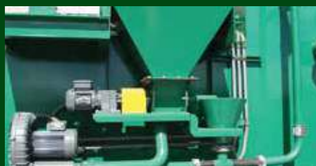
Dry flocculent powder is transferred to the wetting operation by a screw feeder and blowing line.
